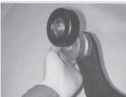
10. The automatic belt tensioner removes the slack from the supercharger belt and decreases boost lag.
