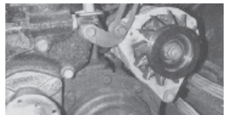
12. The original alternator pulley must be carefully removed. This can be done on the car if you have access to an impact wrench. Otherwise, it's a good idea to remove the alternator and have the pulley removed and replaced with the new ribbed pulley by a shop.
